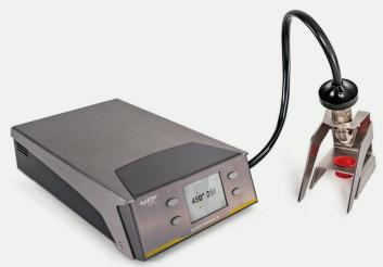
sure-technology. This allows reliable dispensing of very small dots and lines of liquid to pasty material either as 1K-type or 2K-type. In addition, a sensor measures the material temperature inside the dispensing pen and the control unit compensates the material-specific change in viscosity. You can add your own material to the already existing material library to define essential material parameter and limit values.
